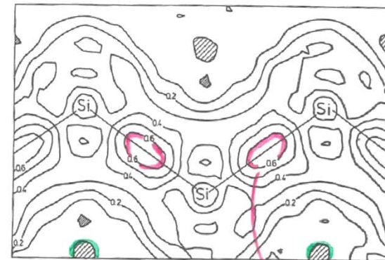
Fig. 1.8. Density of valence electrons in a typical ionic crystal (NaCl) and in a typical covalently bound crystal (Si) [1.2, 3]. One clearly sees the concentration of charge along the bond between Si atoms, whereas in the ionic bonding, the electrons are almost spherically distributed around the ions
