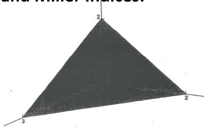
Figure 20 This plane intercepts the a, b, c axes at 3a, 2b, 2c. The reciprocals of these numbers are \frac{1}{3}, \frac{1}{2}, \frac{1}{2} . The smallest three integers having the same ratio are 2, 3, 3, and thus the Miller indices of the plane are (233).
